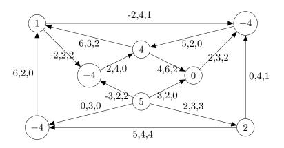
**Solution:** Residual graph is created by keeping edges e with nonzero u(e) - f(e) and adding reverse edges if f(e) > 0. In order to find a negative cycle, we only need to know the cost. It is depicted in in bold.
